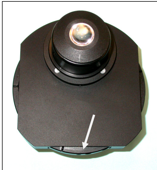
Fig. 16: Combination condenser with rotating disc (arrow).
