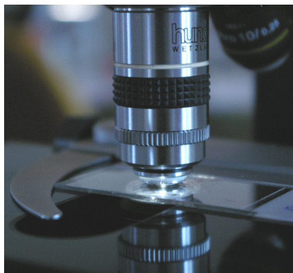
Fig. 4: Objective Plan 100/1.25 – 0.60 Oil with iris diaphragm.
